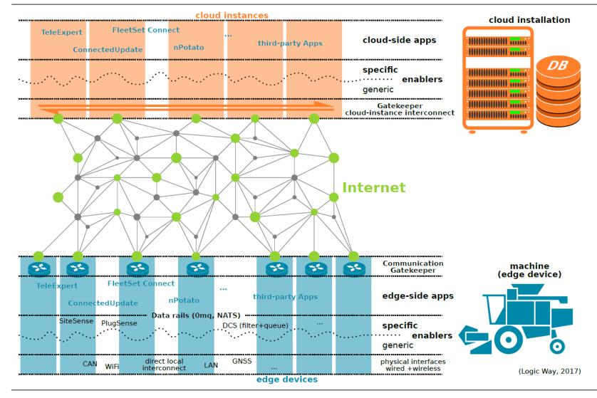
Due to the poor network coverage in rural areas especially in eastern Germany the data processing is divided into cloud and edge applications.
